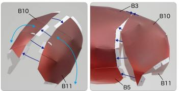
Attach B12 to the body. Glue B13 to B10 and B11, and the body is complete.
